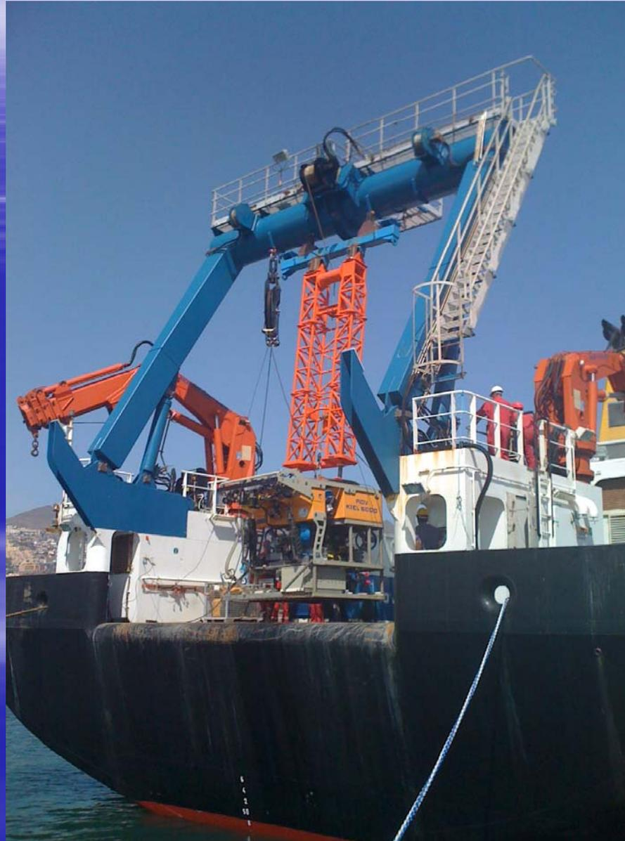
Original fame hanging arrangement with gantry in the inboard position
